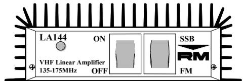
The LA144 is a wideband compact amplifier for the VHF band; covering from 135 to 175 Mhz. Output is nominal 60W at full power (70W max).
