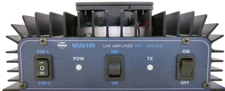
The MUA100 is a wideband compact amplifier for the UHF band; covering from 405 to 480 MHz. Output is nominal 100W at full power (115W max).
